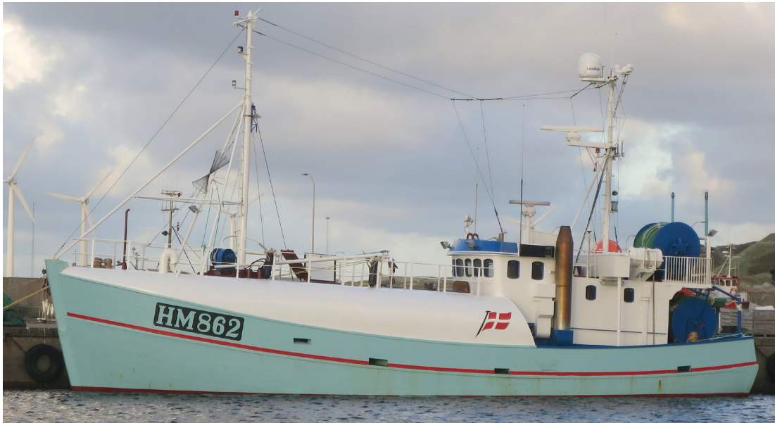
Fig. 52: HM 862 'Christina Paulsen of Hanstholm' is one of the unilaterally specialized 100 GT anchor seiners operated by the Fishing Culture 6 crew of 3 or 4 share fishers. The wooden boat is constructed in Hvide Sande in 1986 and has been owned and operated as 'Ralima of Hanstholm' by a family and its local crew from Thorupstrand until 2025. At that time it was bought by two young fishing families, who sold their shares in the 123 GT Flyshooter and trawler L 654 'Pia Glanz of Thorsminde' with the aim 'to get more freedom' and less fuel consumption by fishing with anchor seine in Skagerrak. Photo: Thomas Højrup, Hanstholm 2016.
