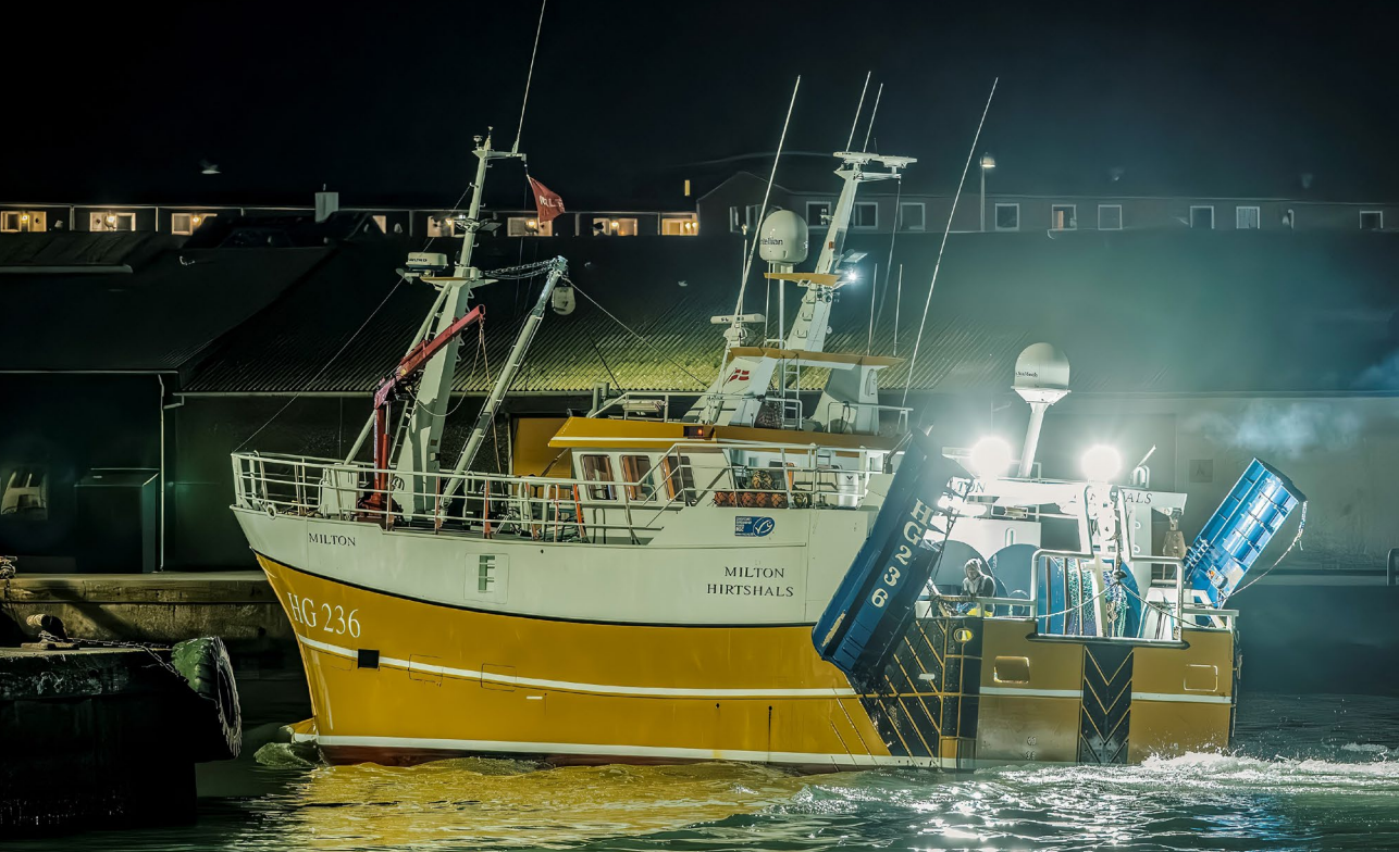
Fig. 55: HG 236 Milton of Hirtshals is a harbour based coastal fishing vessel, measuring 17-meter length and 93 GT. The fishing family got the hull constructed in Poland at request and design of Vestværftet in the North Sea harbour Hvide Sande in 2017. It became equipped with machines, winches, cooling system, navigation instruments etc. by the local marine shops in Hirtshals, fit out for longlining, demersal trawling, pelagic trawling, gill-netting and other fishing methods, which might show up as relevant for a variable and full annual cycle of share-organised fishing in Skagerrak. The skipper's ambition was to develop a small-scale vessel to the broadly complex, versatile mode of operation, that could inspire other share-fishermen to order similar boats in order to strengthen the harbour based coastal fishing fleet in Hirtshals and recruit new generations for this kind of fisheries. In March 2026, the vessel was bought by a younger fisherman in Hanstholm, who sold his boat share in the 50 m long and 1.306 GT pelagic trawler Lingbank: "It is a completely different ship than the old Lingbank, much smaller and thus far less financial pressure, says Jonas Rasmussen, who is delighted to have his foot on his own deck again." https://ligeber.nu/thy-mors/nybeder/aktuelt 19. marts 2026. Photo: Jens Kranen Photography.
