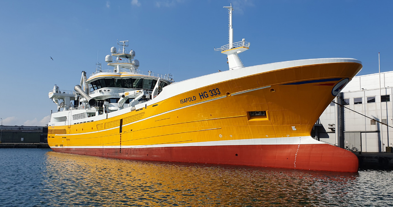
Fig. 40: The 2022 version of the family owned 4750 GT pelagic trawler and purse seiner HG 333 'Isafold of Hirtshals' is landing its catch to Scandic Pelagic in Skagen. In contrast to the Dutch pelagic factory trawlers, the Danish pelagic fishing vessels store and transport the catch in Refrigerated Salt Water tanks aboard the boats aiming to land it in a hurry to the fishing companies' processing factories in Skagen and other Nordic fishing harbours. Photo: Thomas Højrup, Skagen 2022.
