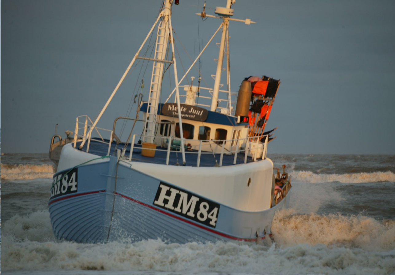
Fig. 36: The typical Fishing Culture 1 vessel HM 84 'Mette Juul' of Thorupstrand' was launched 2002 as a new 22 GT combined gillnet and anchor seine vessel, able to be launched from and land at the open beach of the landing site. Its crew is catching all kinds of demersal and benthic fish species available at the distinct seasons during a full year circle. The flexibility of the boat's clinker-craft oak hull makes it well-suited for beach landing and launching in Thorupstrand and Løkken. The practice of building and using Nordic clinker-crafts is inscribed by UNESCO on the Representative List of the Intangible Cultural Heritage of Humanity. Photo: Thomas Højrup, Thorupstrand 2011.
