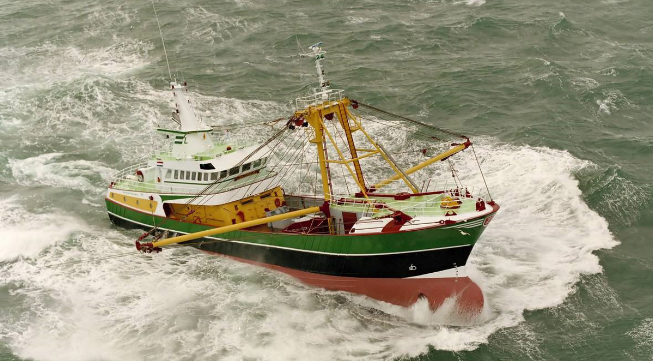
Fig. 44: In 2017–2018 the Hakvoort Brothers from Urk got the new beam trawler UK 46 constructed by the Damen Maaskant Shipyards Stellendam. The picture was posted by Michelle Howard May 11, 2017, at the shipyard's homepage to illustrate the well proven Damen Maaskant design. The vessel is 41 meters in length and propelled by a type 12 DZC main engine from ABC, delivering 1999 hp. Photo: Damen Shipyards.
