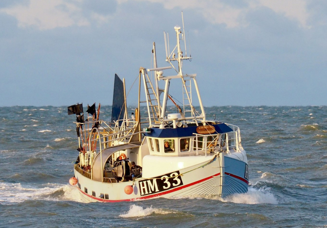
Fig. 35: Operated by 3 share organised coastal fishers, the 27 GT combined gillnetter and anchor seiner HM 33 'Kikani of Thorupstrand' is returning home with gillnet-caught cod from the stone reefs in Jammer Bay a windy day in January 2023. Kikani was constructed and launched at the landing site of Slettestrand in 2017 and got its name from the boat-share owner family as a condensation of the married couple Kirsten and Karsten Nielsen. Photo: Dan Sejbjerg, 2023.
