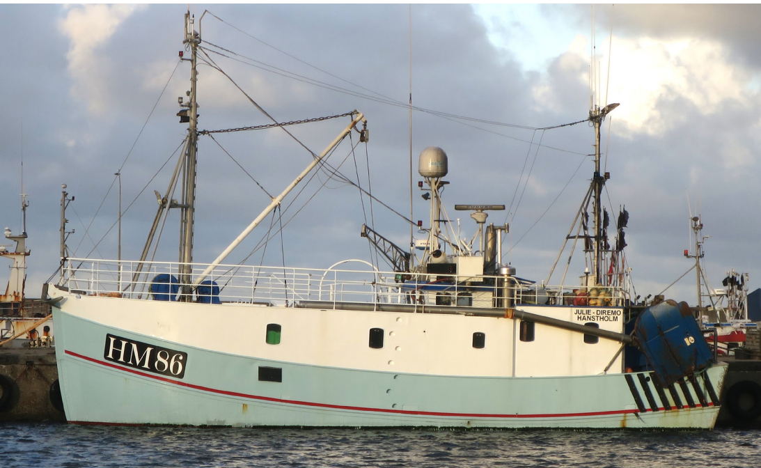
Fig. 51: Father, son, and a third share fisher is a typically crew size when a GT 20 coastal vessel combining single trawling and gillnetting is conducting inshore fishery in Skagerrak. HM 86 'Julie Diremo' was constructed in 1982 for coastal fishing from a harbour. The boat underwent succeeding modernizations, became bought and reshaped by a fishing family in Thorupstrand and operated from Hanstholm, where the picture of this typical Fishing Culture 4 vessel was taken in 2015. Photo: Thomas Højrup.
