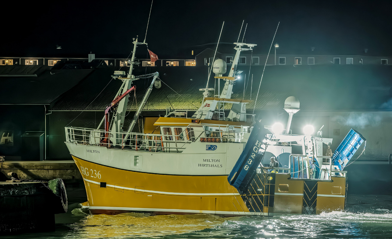
Fig. 55: HG 236 Milton of Hirtshals is a harbour based coastal fishing vessel, measuring 17-meter length and 93 GT. The fishing family got the hull constructed in Poland at request and design of Vestværflet in the North Sea harbour Hvide Sande in 2017. It became equipped with machines, winches, cooling system, navigation instruments etc. by the local marine shops in Hirtshals, fit out for longlining, demersal trawling, pelagic trawling, gill-netting and other fishing methods, which might show up as relevant for a variable and full annual cycle of share-organised fishing in Skagerrak. The skipper's ambition was to develop a small-scale vessel to the broadly complex, versatile mode of operation, that could inspire other share-fishermen to order similar boats in order to strengthen the harbour based coastal fishing fleet in Hirtshals and recruit new generations for this kind of fisheries. In March 2026, the vessel was bought by a younger fisherman in Hanstholm, who sold his boat share in the 50 m long and 1.306 GT pelagic trawler Lingbank: "It is a completely different ship than the old Lingbank, much smaller and thus far less financial pressure, says Jonas Rasmussen, who is delighted to have his foot on his own deck again." https://ligeber.nu/thy-mors/nybeder/aktuelt 19. marts 2026. Photo: Jens Kranen Photography.
