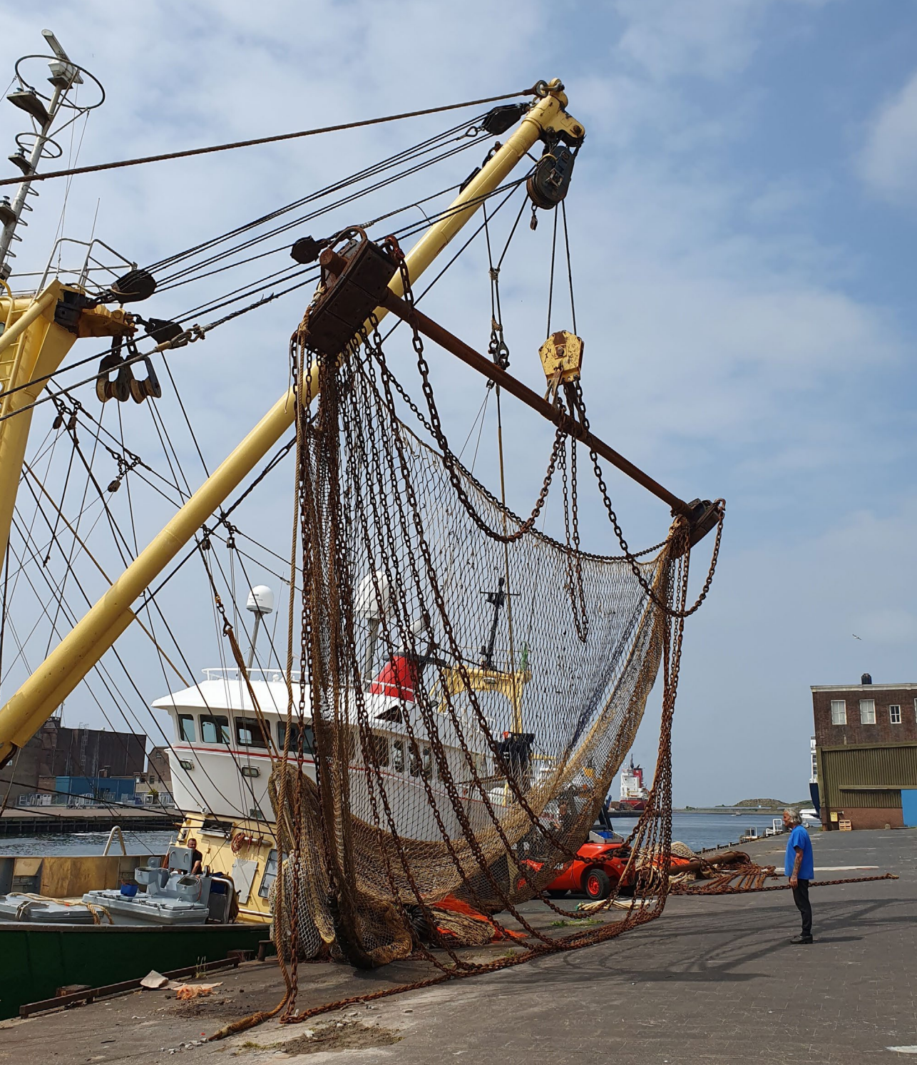
Fig. 43: A beam trawl with 10 heavy steel chains is lifted onto the deck before departure to the fishing banks. The boat drags two of these beam trawls, one on each side of the vessel. Photo: Thomas Højrup, Ijmuiden 2023.
